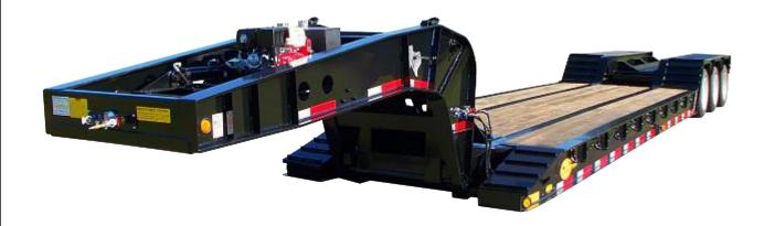
Viking's Hydraulic "Detach" trailer is a real workhorse designed for heavy hauling and simplicity of operation. Two 8" hydraulic rams provide plenty of lift capacity coupled with the power & speed of the 11hp Honda® Engine/pump located in the neck. Fixed front ramps and a heavy 4 beam frame give you lots of strength and a carefree long life. Whether you haul construction equipment or any other drive on load, The Viking "Detach" is the trailer for you. Capacity: 135,000 lb. GVWR.
