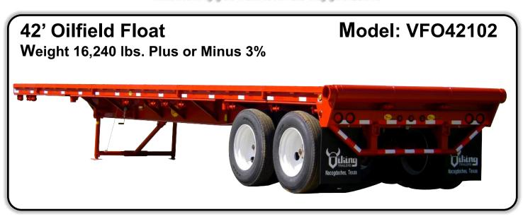
For use in the oil and gas industry, The Viking 42' Oilfield Float provides quick and easy loading with retractable landing gear and pick-up eye for winch use. The heavy duty 8-5/8" tail roller assembly handles the heavy loads and designed with service in mind. The bearings are replaceable and greaseable. The 42' Oilfield Float makes it easy to get around worksites and will hold up to the task. This trailer is built Viking tough! Capacity: 100,000 lb. GVWR.
