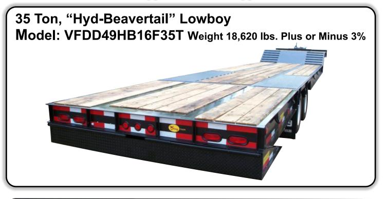
The 35 Ton Hydraulic Beavertail is designed for loading and unloading a variety of heavy equipment. The full width hydraulic apron raised and unfolds and provides a full width loading ramp surface allowing all types of wheel and track machines to be loaded and unloaded safely. Available with a hydraulic winch to assist in loading damaged and non working equipment. Popular in the equipment rental business the Viking 35 Ton is a must have to get the job done. Capacity: 88,000 lb. GVWR.
